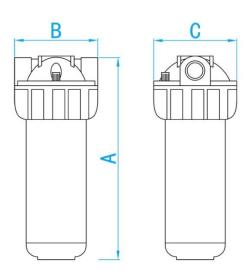
\* Filter cartridge can be used to filter impurities larger than  $5\mu m$  in size.
